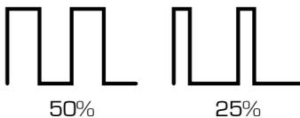
Figure 11-4: Square wave with 50% and 25% duty cycle.
